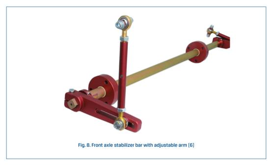
In the discussed solution, the arms are made as separate elements of rectangular cross section. The material used for the arms is AA 6061-T6 high-strength aluminum alloy [7]. This contributes to reduced weight while maintaining its high strength characteristic.
